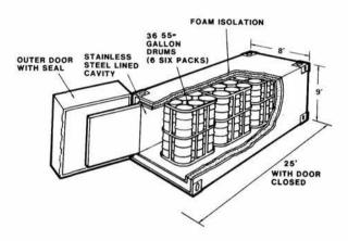
STEEL-FOAM-STEEL walls provide TRUPACT's protection to cargo.
